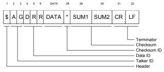
Checksum: Checksum is the exclusive – OR between "\$" and before the "\*"/ The hex value of the result are converted to ASCII characters.
