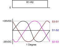
External heading signal for back up at auto steering unit.
